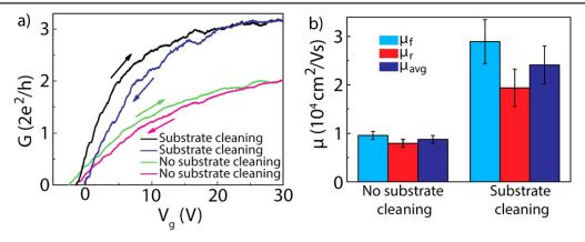
**Figure 3.** (a) Conductance curves  $G(V_g)$  obtained from samples without and with substrate cleaning. Forward and reverse sweep direction are indicated with arrows. Samples have been evacuated for ~60 h before cool down. (b) Forward, reverse and average mobility with and without substrate cleaning. Values are averages obtained from fits to conductance curves of individual devices. Error bars indicate standard deviation.
